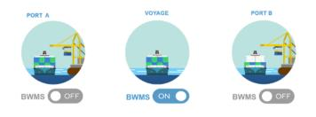
Container ships have a very suitable profile for the Bawat BWMS because they have a high-powered main engine and the amount of ballast water that needs to be exchanged is relatively small. The system is designed to fulfil the actual needs for treatment of ballast water resulting in a small footprint. The utilization of waste heat to drive the BWMS, no filters and no consumables makes OPEX for ship owners negligible.
