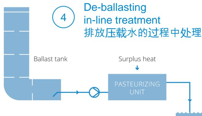
The Bawat BWMS can be applied in different configurations
